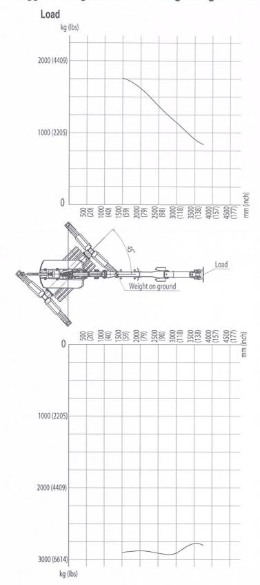
4. On tracks - forward DXR300 - weight on ground will appear on front end of both tracks.
